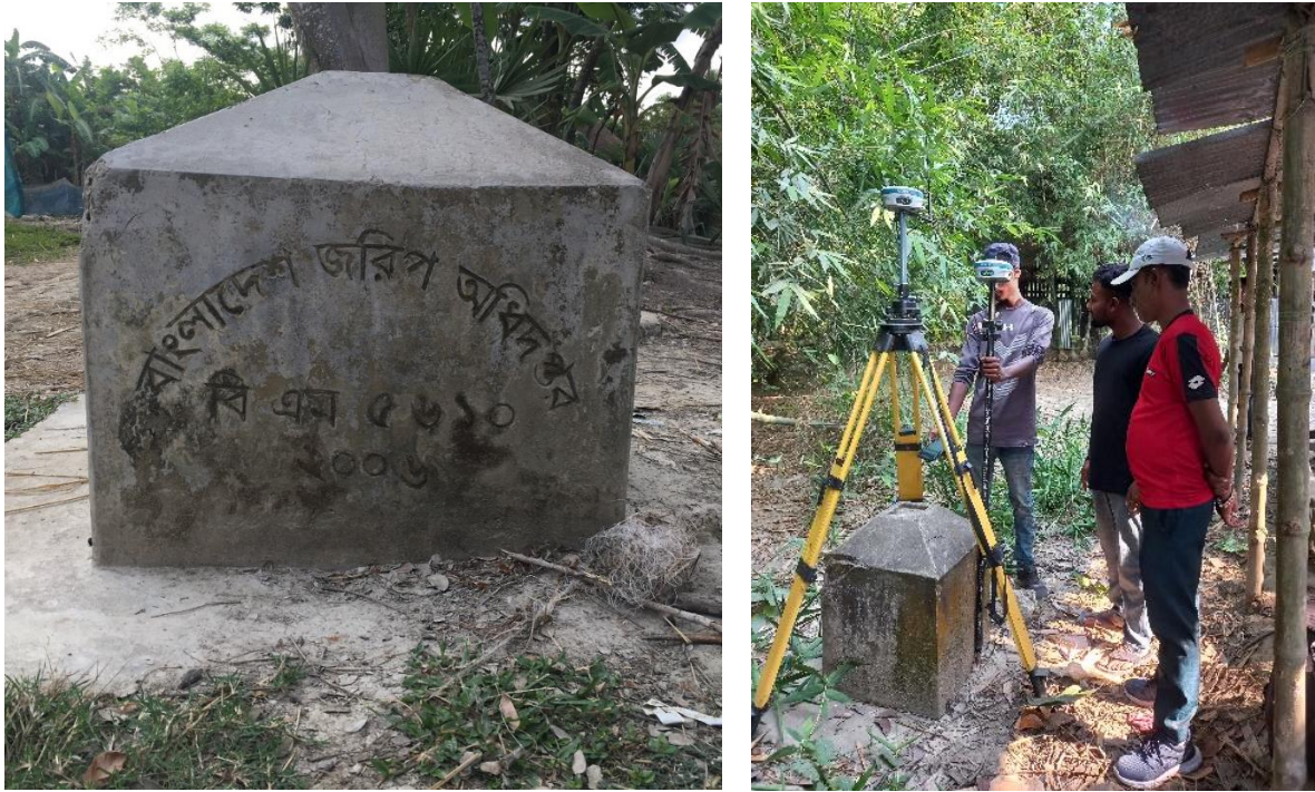
Figure 6.13: Survey of Bangladesh benchmark and base station setup with Base RTK
