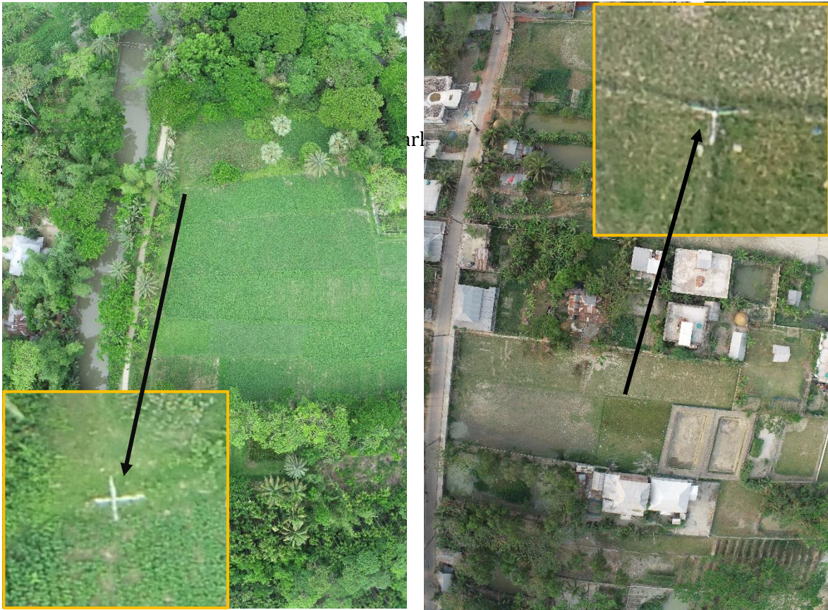
Figure 6.16: Cross mark for GCPs
